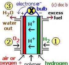
oxygen + polymer hydrogen platinum electrolyte platinum catalytic proton catalytic cathode exchange - anode electrode membrane electrode
